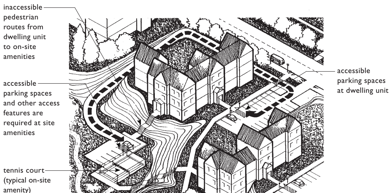
In Some Circumstances, Site Access by Vehicle May Be Acceptable
