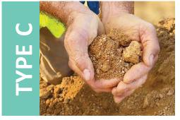
Unconfined compressive **strength of 0.5 tons** per square foot or less.
