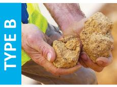
Unconfined compressive **strength greater than 0.5 tons** per square foot but **less than 1.5 tons** per square foot.
